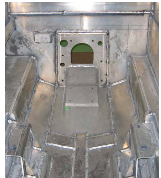
Template welded to the aluminum hull.
