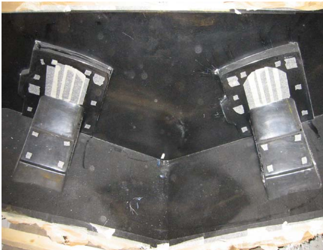
Twin-installation template adapter part for the boat mould.
